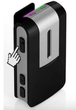
**Step 2:** You can now use the StreamLine Mic as a remote microphone with a range of up to 20 meters. The sound from the speaker wearing the mic will be streamed into both hearing aids.
