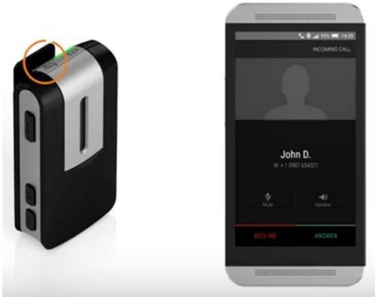
**Step 5:** When the call is accepted on the phone or via pressing the MFB, the call is automatically streamed into both hearing aids. The call can be made completely hands-free.
