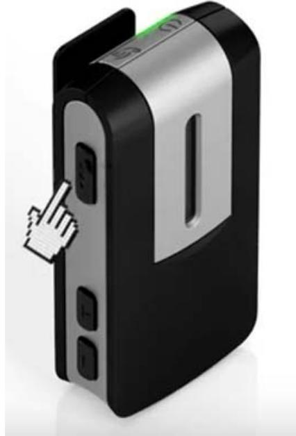
**Step 2:** With the MFB, you can toggle between Bluetooth Streaming Mode and Remote Microphone Mode. The status indicator shows you different uses in different colors.
