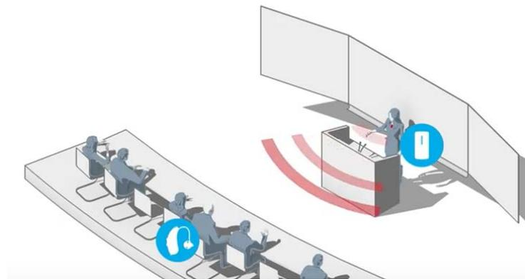
**Step 3:** When used as a remote microphone, the StreamLine Mic should be worn vertically to maintain microphone directionality.
