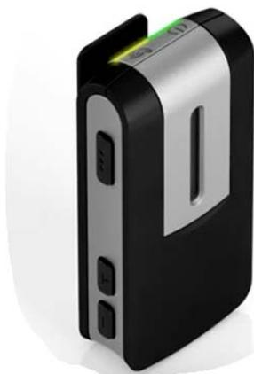
Pairing is successful as soon as the yellow light stops flashing and stays on.
