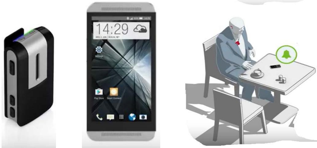
**Step 3:** To answer the call, use your phone as usual or briefly press StreamLine Mic's multi-function button (MFB). The phone call is streamed automatically to both ears and can be completely hands-free. The status indicator stays green while the phone call is active. To end the call, press the MFB or use your smartphone.
