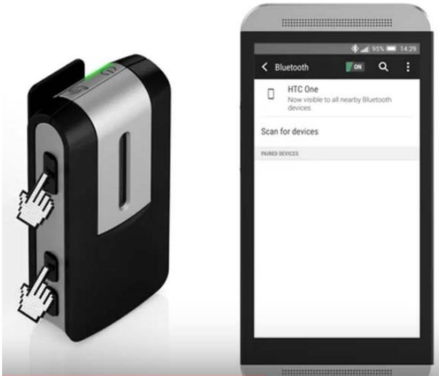
**Step 4:** You have 3 minutes to complete the pairing. Select StreamLine Mic from the list of detected devices on the Bluetooth menu. If requested, enter the PIN 0000. A solid green power indicator and solid blue status indicator verify connection to smartphone is successful.
