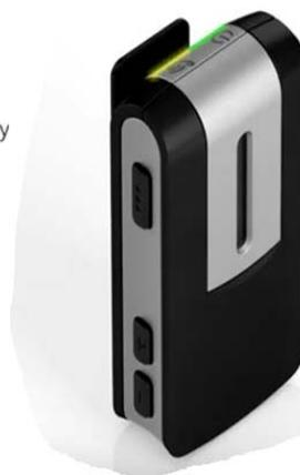
The status indicator starts flashing yellow which shows that the pairing process has started automatically.
